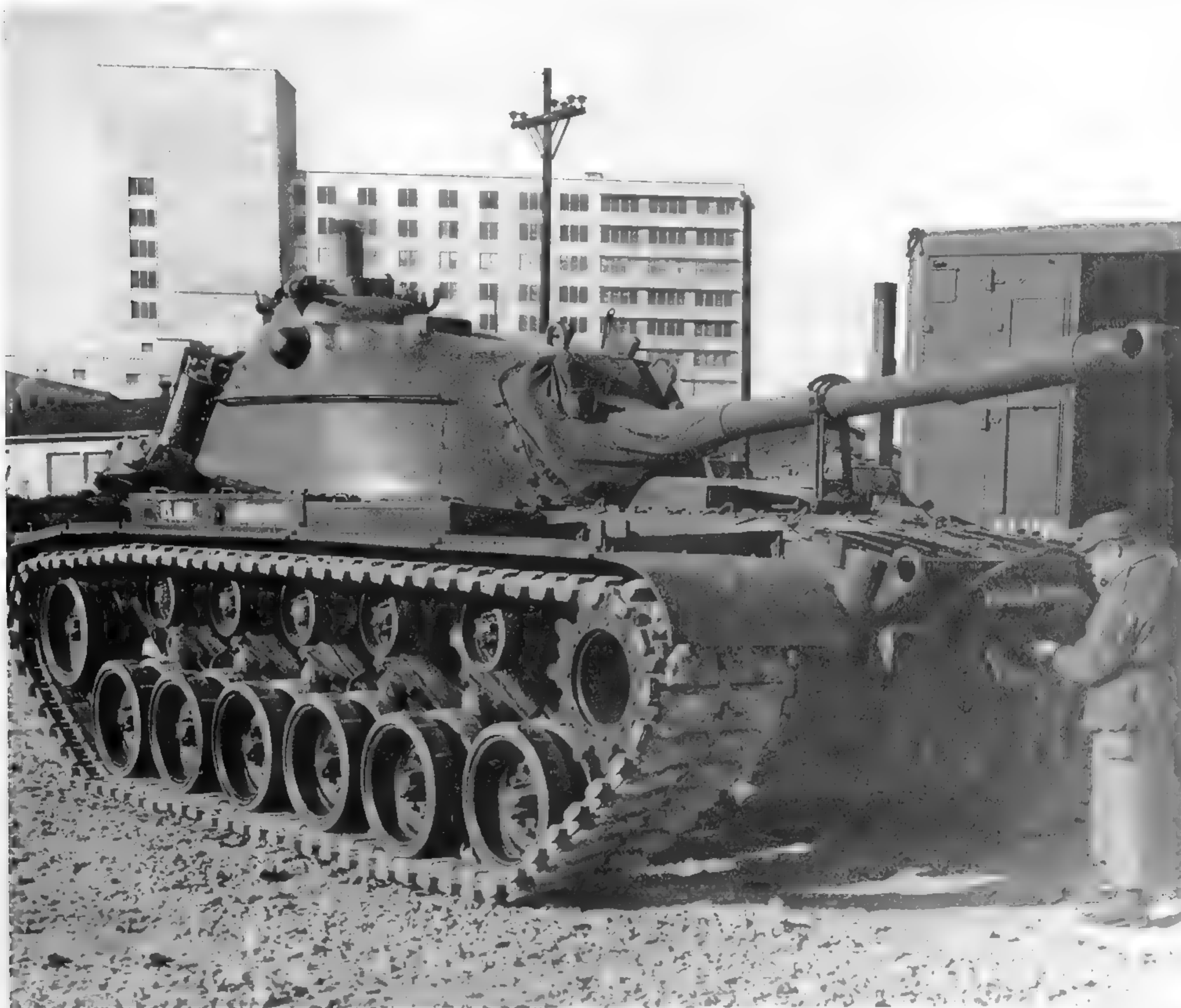
A technician checks the telephone installation on the rear of an M48. The telephones, housed in a box on the hull rear, allowed infantryman on the ground to talk to the tank crew under combat conditions. The tank is prepared for travel, with its turret rotated to the rear and main gun in its travel lock. (Photo courtesy of the Patton Museum)
